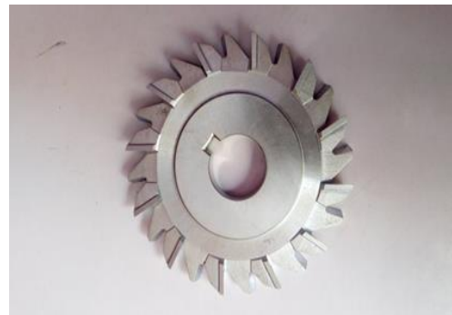
Figure.10. Fabricated piece of plain milling cutter
