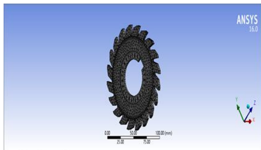
Figure.6. Mesh model of plain milling cutter
